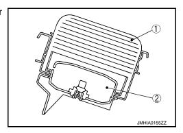
Passenger air bag inflates by breaking instrument panel surface
