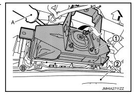
4. Remove passenger air bag module from instrument panel assembly according to numerical order 1→2 indicated by arrows as shown in the figure.
