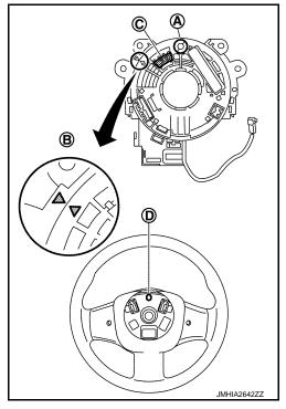
Fix the driver air bag module harness to the harness fixing hook (A).
