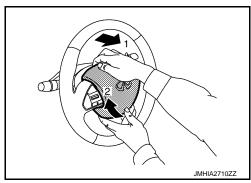
3. Disconnect driver air bag module harness connectors (B) and horn switch harness terminal (A).
