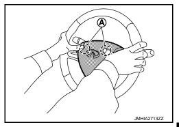
• Press driver air bag module lower (A) until it snaps into place with a clicking sound.
