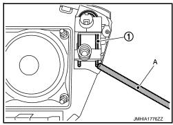
Lift up driver air bag module lower side from vehicle front to upwards while pulling driver air bag module upper side according to the numerical order 1→2 as shown in the figure, and then pull out driver air bag module.
